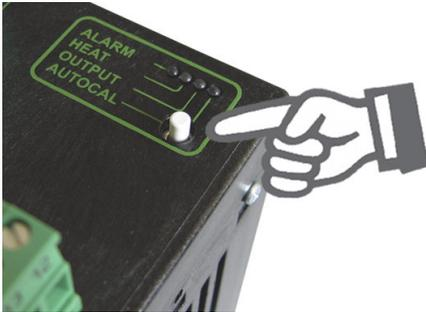
The automatic calibration process takes about 10...15 seconds. The heatsealing band is not heated during this process.
