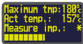
The heating and control process can thus be observed at any time. The RESISTRON monitoring device RESM-5 additionally supplies an electrically isolated, analog 0...10VDC
