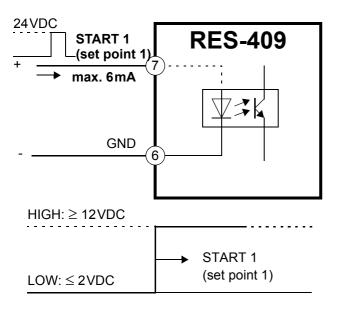
The set point selected for the heatsealing temperature must be greater than 40 °C. If not, the heatsealing band is not heated ("HEAT" LED blinks).
