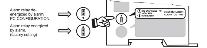
If the jumper is not inserted, the fault relay is permanently energized (fault contact between terminals 13 and 14 closed). The other controller functions (e.g. heatsealing band heating, AUTOCAL etc.) are not affected.
