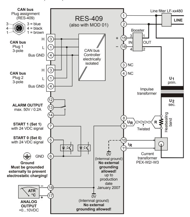
The START 0 and START 1 functions at terminals 5 and 7 are only available on controllers manufactured as of February 2007.
