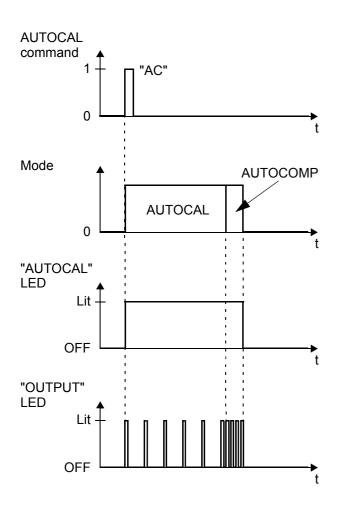
The "OUTPUT" LED blinks repeatedly while the "AUTOCOMP" function is running and the actual value output (terminals 17+18) is set to 0...3°C (corresponds to approx. 0VDC).
