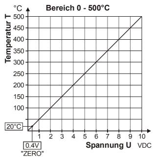
Only the 300°C and 500°C temperature ranges appear at this actual value output. If a temperature range of 200°C is set with CAN message address 8 ("Alloy/range"), it appears at this output in the 0...300°C range. A 400°C temperature range is indicated as 0...500°C.
